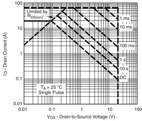
$^*$  V<sub>GS</sub> > minimum V<sub>GS</sub> at which R<sub>DS(on)</sub> is specified **Safe Operating Area, Junction-to-Ambient**
