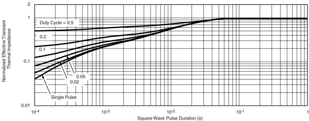
Normalized Thermal Transient Impedance, Junction-to-Case
