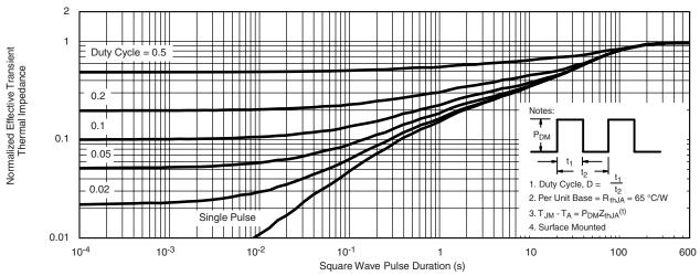
Normalized Thermal Transient Impedance, Junction-to-Ambient
