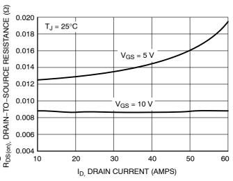
Figure 3. On-Resistance vs. Gate-to-Source Voltage
