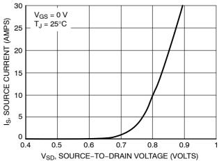
Figure 10. Diode Forward Voltage vs. Current
