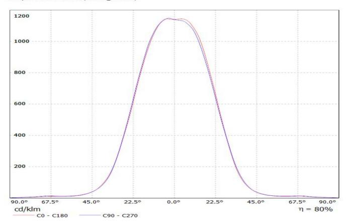
Luminaire: LEDiL Oy CA12804\_EVA-W\_(MK-R) Eff. 79,8% Lamps: 1 x Cree MK-R (356Im@250mA)
