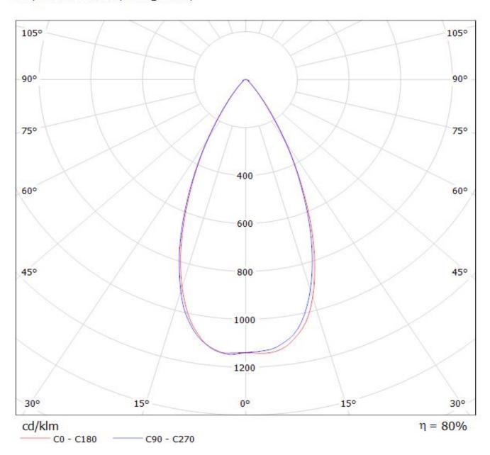
Luminaire: Ledil CA12804\_EVA-W & CP12820\_EVA-W (Luxeon M) Efficiency=80% Lamps: 1 x Luxeon M (362Im @ 250mA)
