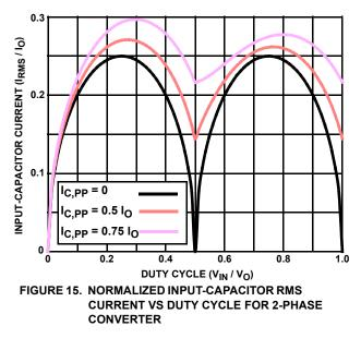
For a two phase design, use Figure 15 to determine the input-capacitor RMS current requirement given the duty cycle, maximum sustained output current ( $I_O$ ), and the ratio of the combined peak-to-peak inductor current ( $I_{C,PP}$ ) to  $I_O$ .
