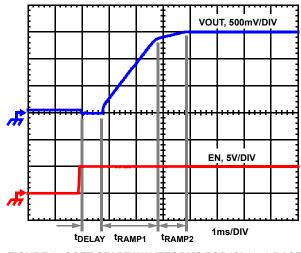
FIGURE 9. SOFT-START WAVEFORMS FOR ISL6559 BASED MULTI-PHASE BUCK CONVERTER
