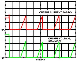
FIGURE 11. OVERCURRENT BEHAVIOR IN HICCUP MODE
