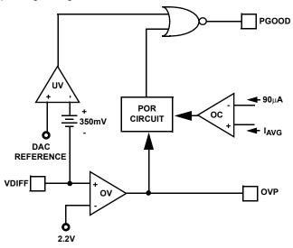
FIGURE 10. POWER GOOD AND PROTECTION CIRCUITRY
