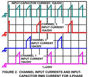
CAPACITOR RMS CURRENT FOR 3-PHASE CONVERTER
